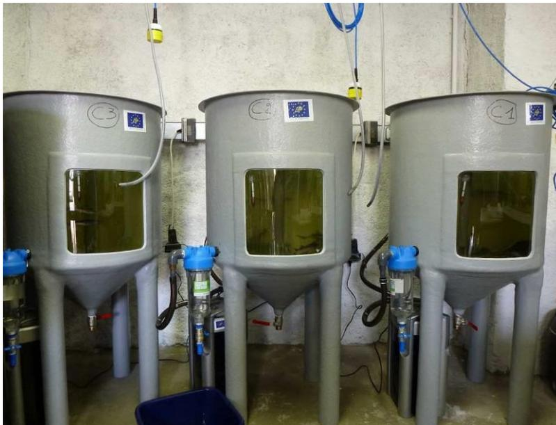
**Figure 14. Cylindroconic tanks to maintain the infested fish. They are equipped with a filter and/or a juvenile collector (Photo: R. Araujo)**
