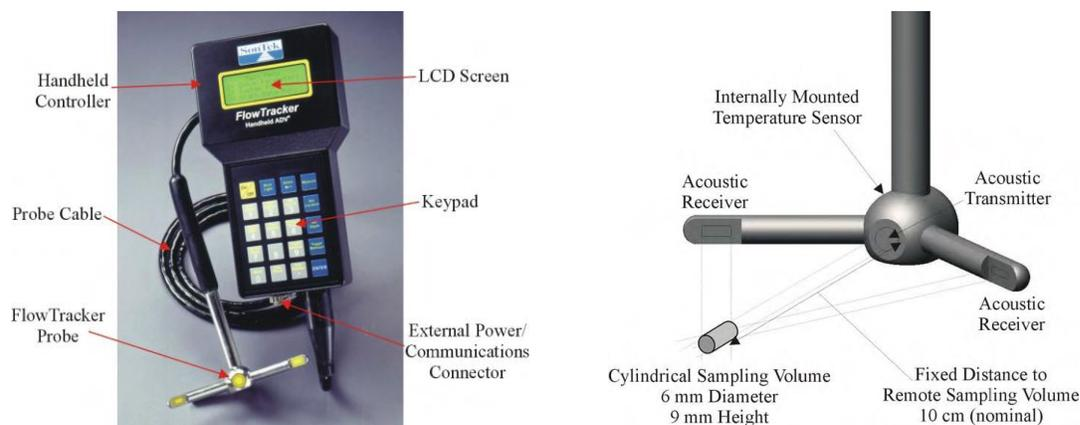
**Figure 27. ADV current meter used for measure water velocity (source: NovoTec)**
