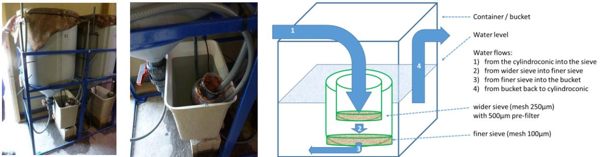
**Figure 16: Juvenile collector system in the cylindroconic tanks (Photos R. Araujo, graph: K. M. Wantzen)**
