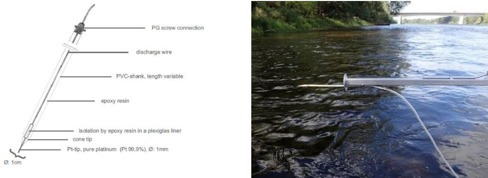
**Figure 30. Device used for Redox Potential (left) and interstitial water measurements (right) Photo: J Soler**
