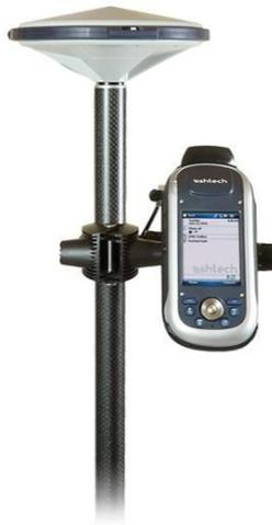
Figure 25. Centimetre GPS used for precise location of mussels. (source bs-tech)
