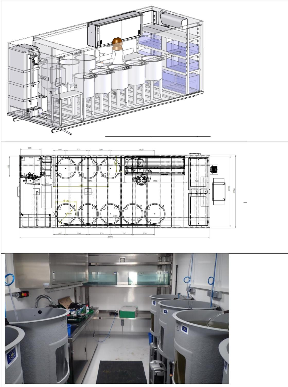
Fig. 5: Above: lateral view, middle graph, plan view of the mobile fish laboratory (design: CASTEX). Below Photograph of the container lab, taken from the entrance (c) M. Sicot).
