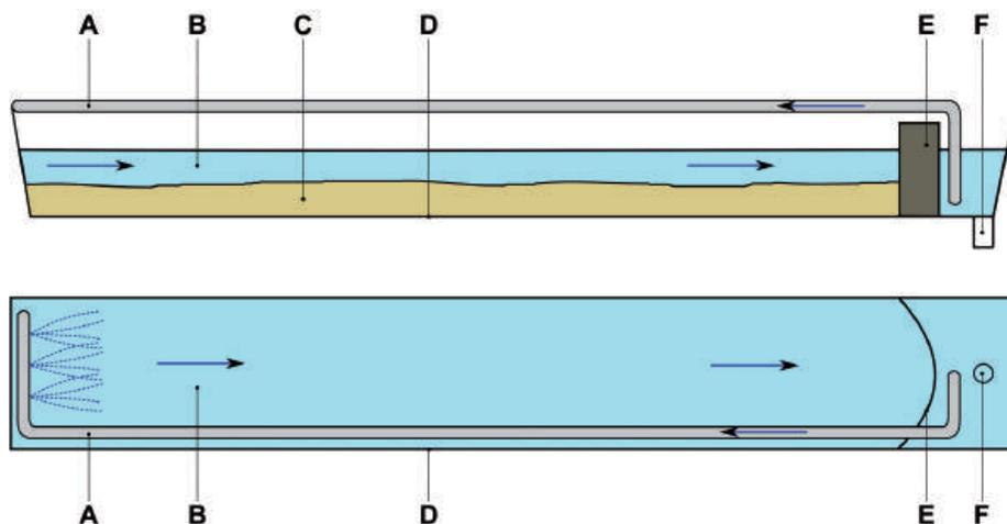
**Figure 19 Artificial flumes. Above, side view; below, top view (A: water return pipe fed by a pump; B: water filtered at 36 µm; C: aquarium substrate; D: plastic tray; E: grille holding the substrate to one side; F: trough purging system). (Source: Freshwater Pearl Mussel Conservation in the Armorican Massif. Programme Report, 2010–2016)**
