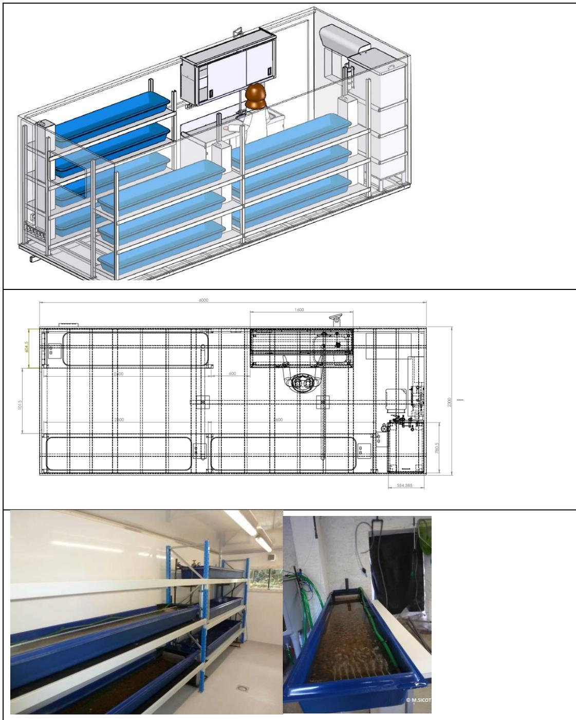
**Fig. 6:** Above: lateral view, centre: plan view of the mobile MUSSEL laboratory (design: CASTEX). Below: artificial flumes.
